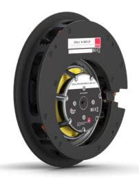
One highly visible and key attribute to the K-60 LP's performance is the complex 3D form of its pressed and anodized aluminum diaphragm. The selection of this material was necessary in to achieve the necessary rigidity for its low profile driver architecture, which also incorporates seven localized stiffening ribs. These not only provide further rigidity but also provide a channel for the voice-coil lead-out wires, allowing for increased excursion. As a direct result of its
